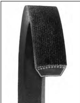
Featuring a rubber impregnated wrapped fabric cover, high modulus polyester cord and specially formulated belt core, The Dayco FHP Utility Belt offers superior performance. Designed for use with fractional horsepower motors utilizing small diameter pulleys, this Dayco FHP Utility Belt delivers extreme flexibility and a smooth, quiet operation over a multitude of fractional horsepower drive applications. **Note: Not for use on clutching drives.**
