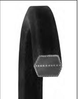
The Dayco Double Angle V-Belt transmits power from either side of the belt. Polyester cords and a durable cotton/ polyester cover delivers maximum strength and length stability while ensuring resistance to heat, ozone, grease, oil and dirt. Specially formulated core compounding provides for long life and high horsepower capabilities. This belt flexes equally well in either direction and provides natural wedging action on both sides for maximum power.
