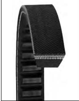
The Dayco Premium Industrial V-Belt's unique construction, which combines the superior flexing of precision molded cogs with the tenacious gripping power of raw edge sidewalls, provides significantly longer belt life without jeopardizing increased horse-power capacity, and/or higher speeds on industrial type drives.
