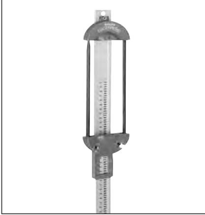
Find the exact Dayco replacement belt instantly. A quick check shows the top width and length/part number of the corresponding Dayco FHP Utility V-Belt or GPL Premium Utility Belt, Industrial A and B Belts, plus 3VX and 5VX Dayco Gold Label® Cogged Belt.
